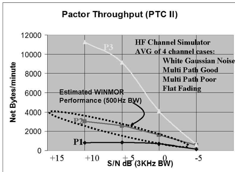
**Figure 4. WINMOR (500Hz) Performance Target Compared to Pactor**
