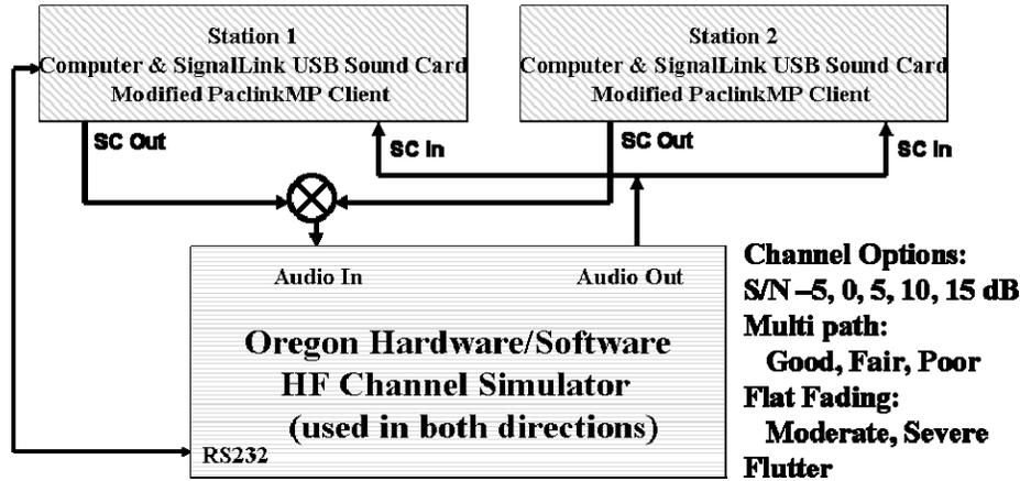
**Figure 3. Protocol Testing Setup using HF Channel Simulator.**
