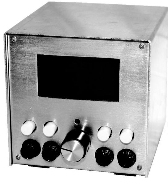
**Photo 1:** Cube prototype prior to application of black powder coating and white silkscreen labeling. Designed as initial companion to NUPSK digital modem, future growth will encompass modem functions and more.
