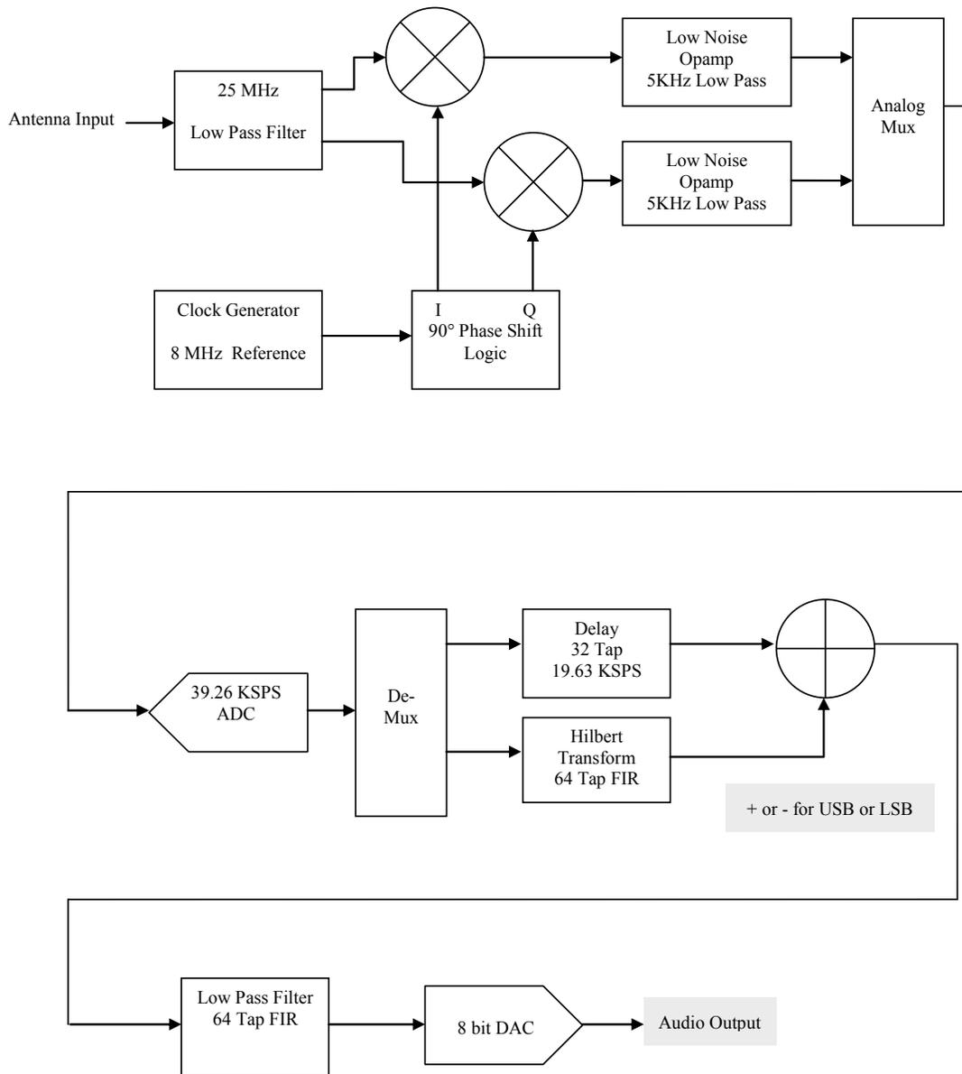
Figure 2: SDR Receiver block diagram.
