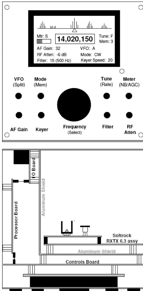
**Figure 4: Front and Top view of the SDR Cube**
