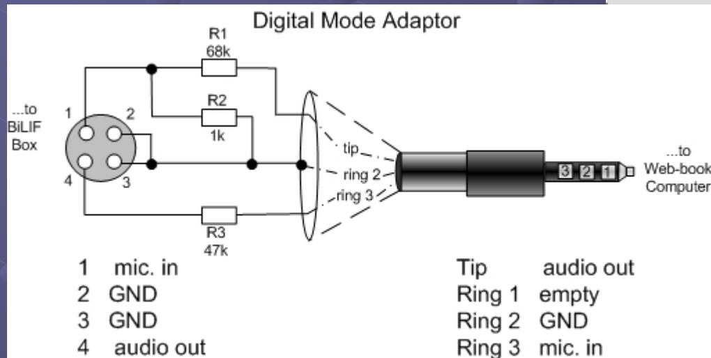
The setup with USB sound cards and Web books requires a special 1 tip – 3 ring plug for the connection to the onboard sound device.
