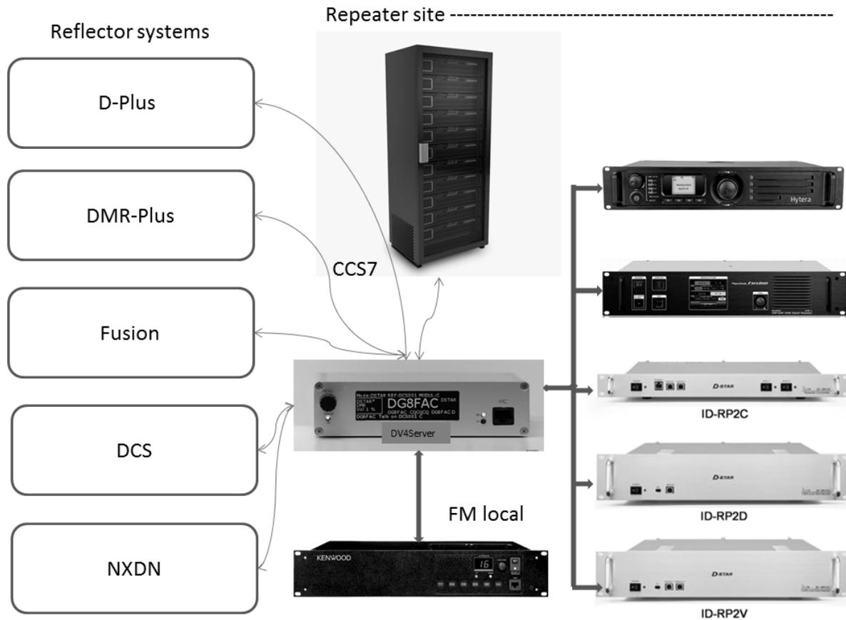
The DV4Server is an optimized embedded LINUX system, which uses the same hardware as the DVhome with AMBE chips, but a different software package.
