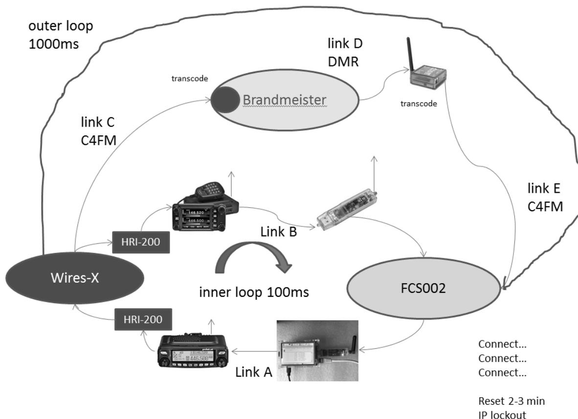
In this example a Raspberry Pi with a DV4mini connects to a room in the Fusion reflector in the DMR Plus system. This acts as a local Hotspot.
