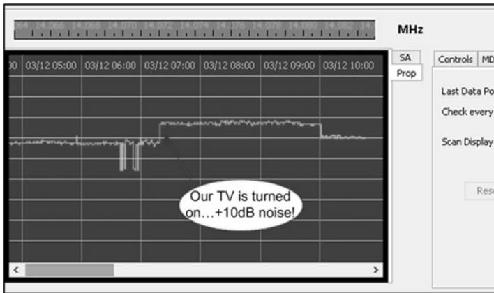
Measuring noise in the environment that surrounds the station is the first task of setting up an RF Propagation monitor. One of the biggest contributors of RF noise is the flat-screen TV. By monitoring the time noise occurs and vanishes one can pinpoint the location of offending units.
