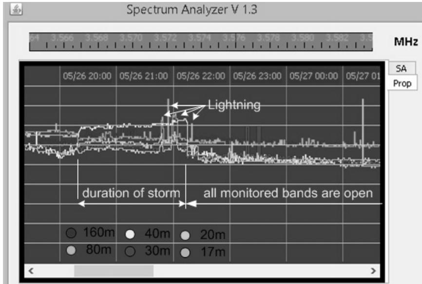
The buildup of energy in the troposphere was visible at least 2 hours before the storm hit (left of the "duration of the storm" marker). During the 2h storm the noise level of the 40m band jumped way up. In this particular storm the lightning passed last, mostly seen in the green spikes (80m). Just after 22:00 a big lightning strike makes even the 17m band jump. At 22:15 the noise of the 40m band drops almost immediately even though the storm was only a few miles away. And then something
