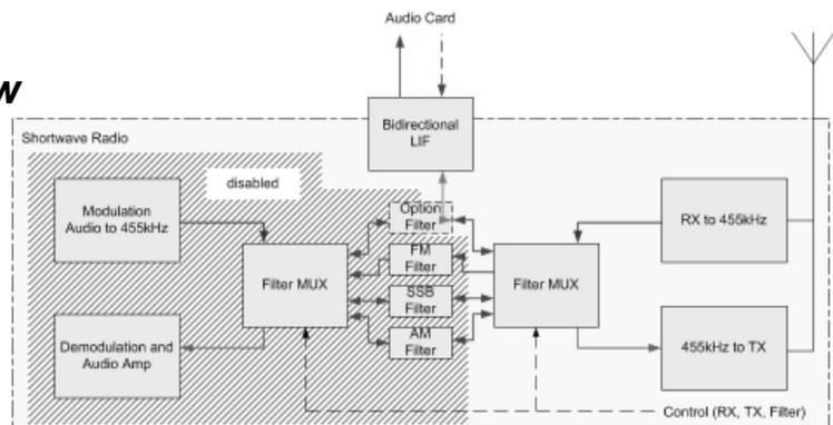
By processing the IF and not base audio, the MDSR software can perform a lot of the functions which most transceivers lack. As a second connection, the CAT cable is required to allow control of all functions of the host transceiver via the MDSR software. Thus, MDSR so completely controls the transceiver that it can be out of reach while operating.
