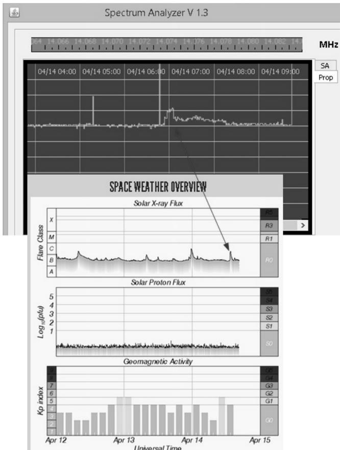
X-Ray Solar Flux hits the ionosphere and causes vibrations in the D-Layer. These changes can be measured and monitored with the single channel RF-Seismograph. In matter of fact the Solar Flux graph on the NOAA website even corroborates the measurement and the time.
