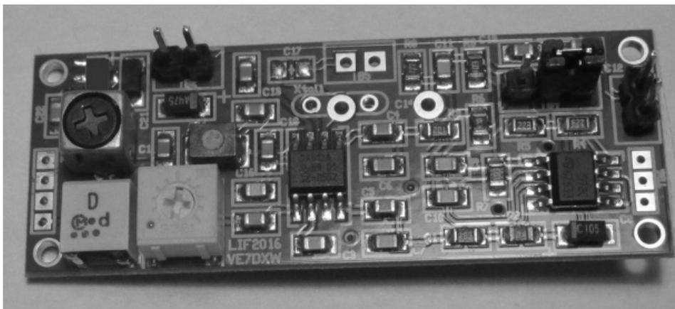
more amateur radio operators. It is mostly SMD and is assembled by robot. The design consists of two layers, and has over 95% ground plane coverage. Now the down-converter hardware is small enough to fit into most transceivers internally. It is actually pin-compatible with the YF-122 crystal filter that
