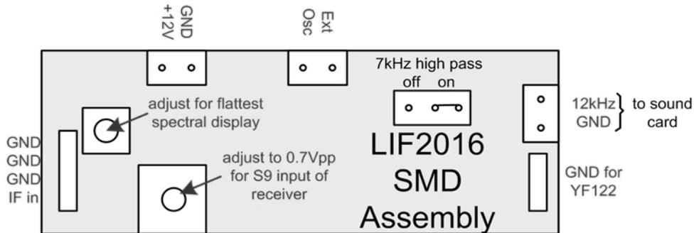
If the unit is placed in a transceiver with a YF-122 option filter, the pin header of the radio fits easily into the left and right PCB holes and slides down for a snug fit. For other receivers, the IF connection has to be made with a jumper. The +12V supply has to be picked off from a suitable spot inside the enclosure.
