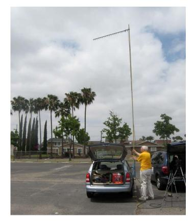
Figure 24 – Bruce KC6DLA adjusts direction for the Field set-up of the 1.2 GHz Transmitting Loop-Yagi Antenna
