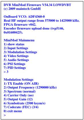
Figure 3 – Typical HyperTerminal Menu Display of the DVB-S Exciter Settings
