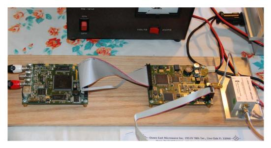
Figure 16 – Breadboard of MPEG-2 Board and MiniMod Exciter Board and the Kuhne 1st-Stage PA (on right side)
