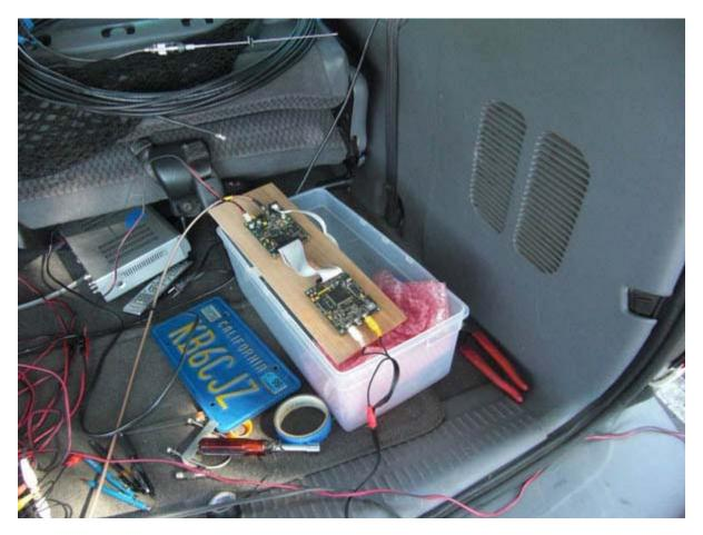
Figure 11 – DATV DVB-S 1 mW Transmitter for 1.2 GHz
