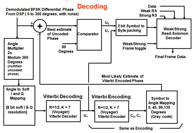
This chart describes how data flows and interacts with various DSP components and processes to implement an 8PSK Pragmatic Trellis Code Modulation Decoder
