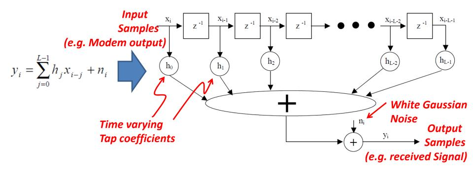
We can use this model and standard CCIR channel definitions to build A very useful DSP based channel simulator application on a PC.
