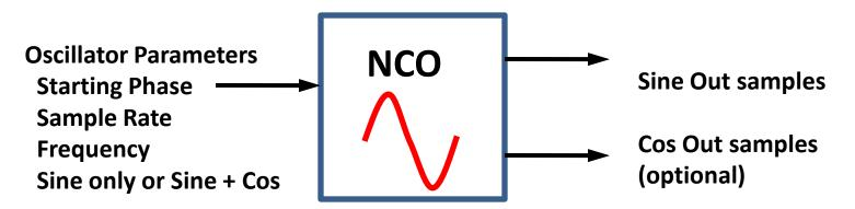
Important note: With double precision floating point we get oscillators with fine frequency resolution and accuracy!
