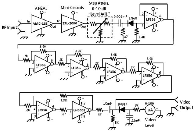
Note: All Buss Connections Bypassed to Ground with 0.1mFC apacitor at the IC Pin.
