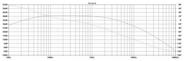
Figure 4: Op amp circuit frequency response.
