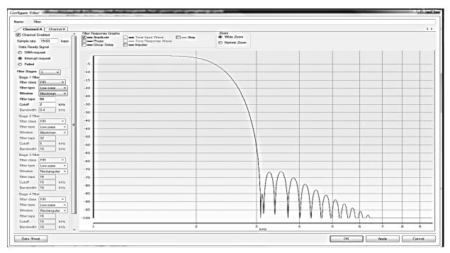
Figure 5: PSoC Digital low-pass filter response.
