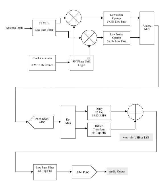
Figure 2: SDR Receiver block diagram.
