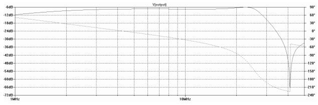
Figure 3: Input RF Filter Response.
