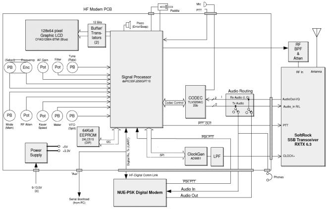
Figure 3: SDR Cube Hardware Architecture
