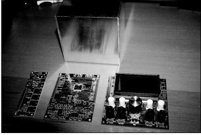
Photo 5: 3-Board Set Cube Custom Aluminum Enclosure (unpainted, before milling) and the three board set of SDR Cube
