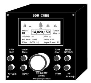
**Figure 1:** Graphic depiction of the completed SDR Cube Transceiver. Dimensioned at 4" x 4" x 4", design contains full user interface, DSP processing, I/O connectors on the rear panel, and 27 in<sup>3</sup> shielded space internally for Softrock.
