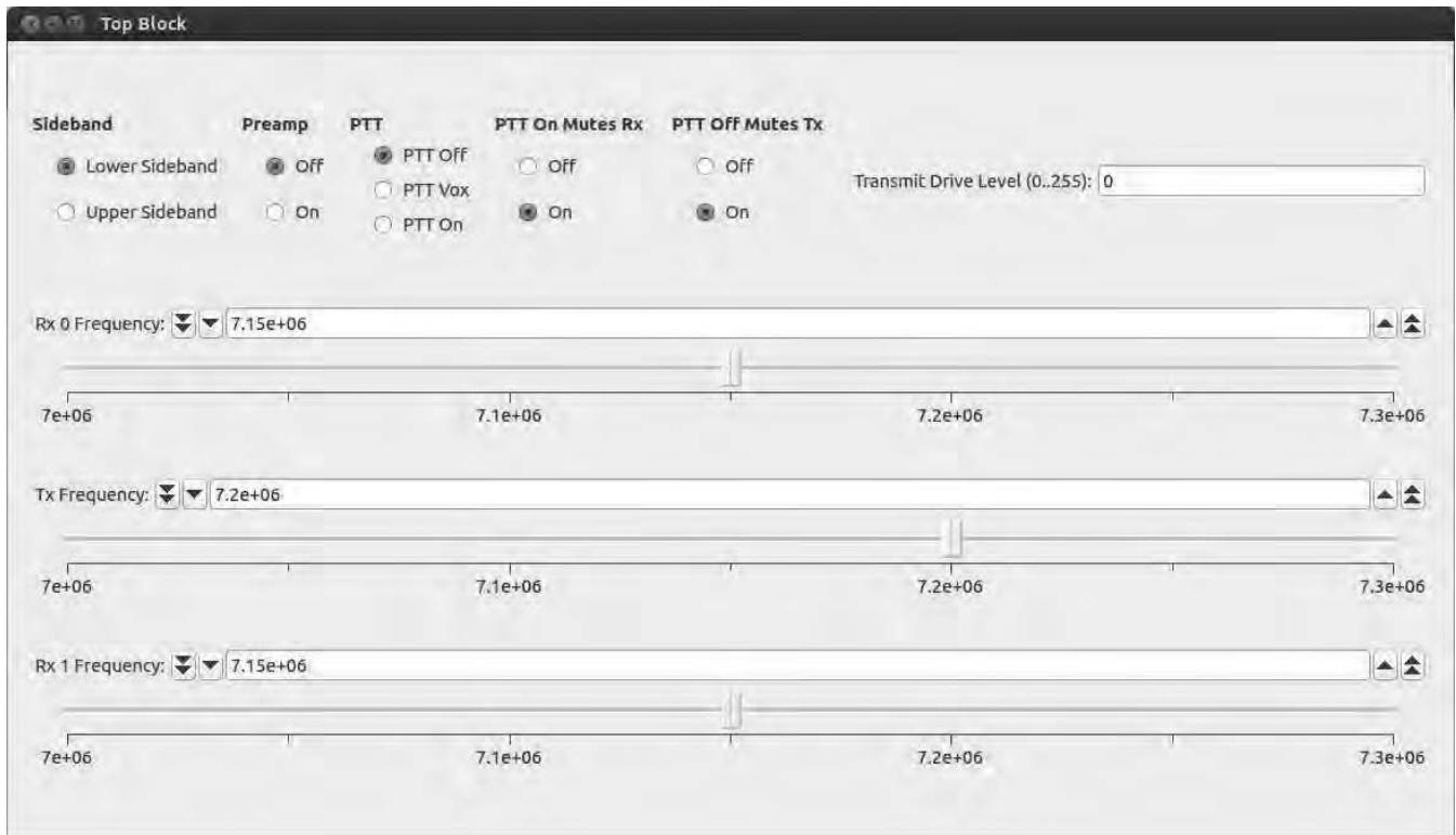
Figure 4 – SSB Receive Control Panel – displays of GUI widgets from SSB Receiver Application of figure 2.
