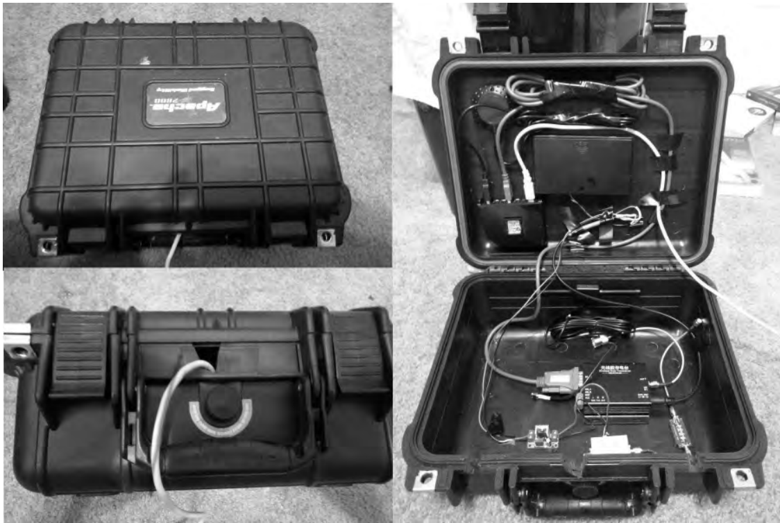
Figure 4: Receive-only mobile setup. The linear regular module (bottom-lower-left), LNA module (bottom-center-left), and 433MHz filter (bottom-lower-right) were not used for the experiments. 8 AA NiMH batteries powered the setup. A USB GNSS receiver provided location information to correlate with received packets.
