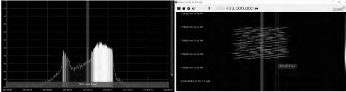
Figure 2: Spectrum analyzer view of the LoRa spread spectrum waveform. Left hand image shows the 125KHz bandwidth of the 300bps LoRa setting, while the righthand image shows a waterfall diagram of the LoRa transmission. While the righthand image partially shows the chirp modulation, the limited sample rate of the RTL-SDR (maximum 3.2Msps) provides a waterfall with a limited resolution, even with the FFT set to the minimum of 512 samples.
