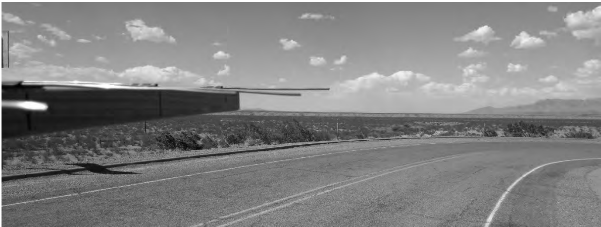
Figure 9: Setting the Ground-Based LoRa Record. The portable Yagi antenna is pointed directly at the horizon, between two groups of mountains.
