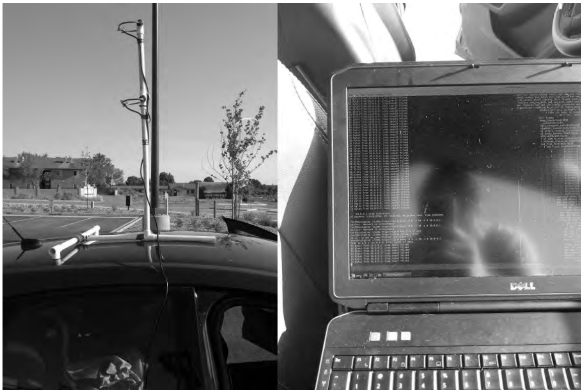
Figure 10: Testing TX/RX Communication in Belen, NM. The vehicle was not moving for these tests, and the mobile double-stacked halo antenna was used.
