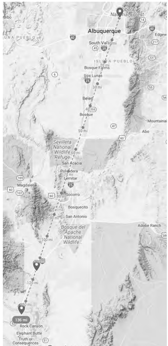
Figure 11: Map showing the location of the transmitting station and the location where the record-setting packet reception occurred. The terrain map shows that the signal path is relatively free of terrain features except for mountains near Socorro. For this particular signal path, computer modeling suggests that the likely propagation path involves diffraction off of the tops of the mountains near Socorro.
