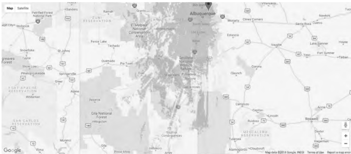
Figure 8: Coverage map for the high-power RX-only setup with the portable Yagi antenna. Green areas indicate areas with an excess link budget of 10dB or more, while yellow areas indicate areas with 0-10dB of excess link budget. The patch of green near Truth or Consequences was the receive location ultimately chosen to set the world record.
