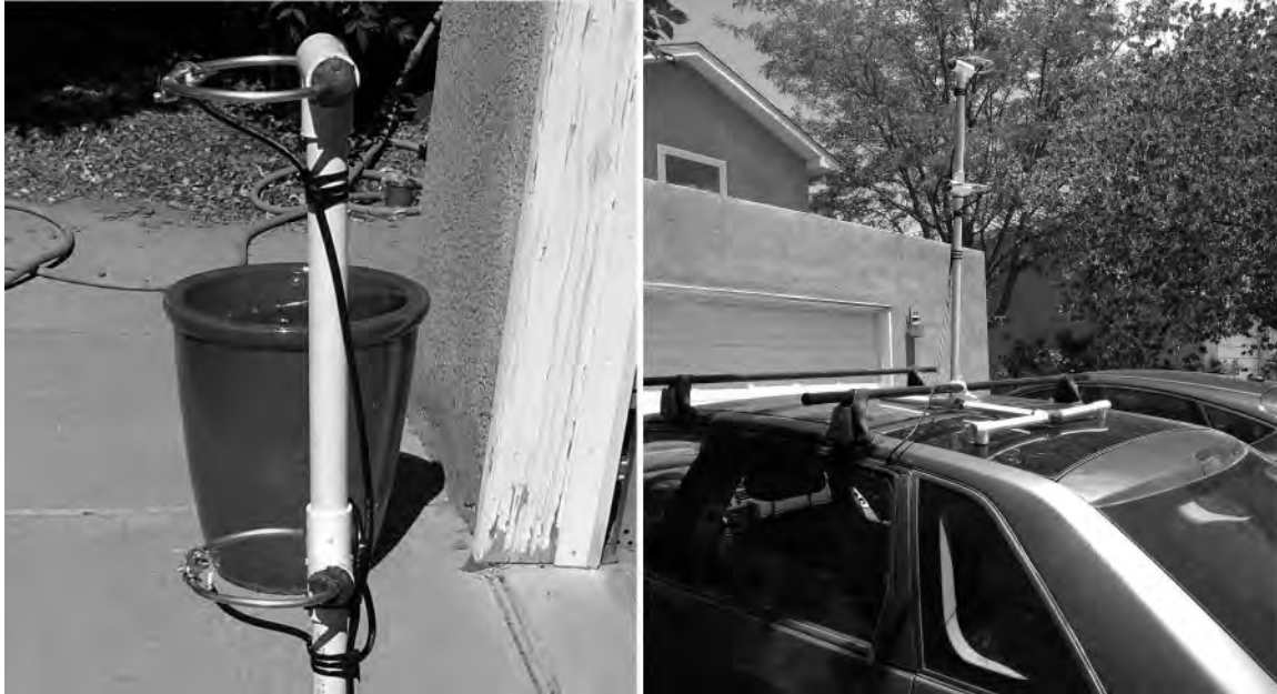
Figure 7: Mobile double-stacked halo antenna. The double-stacked halo antenna successfully received packets while the car was traveling at normal highway speeds down I-25S.
