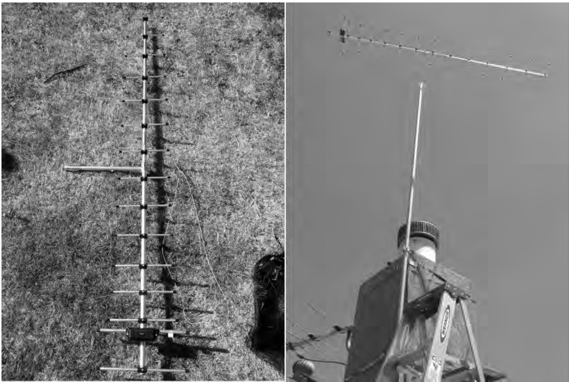
Figure 5: A Diamond 430s15 base station antenna was used for all the LoRa communications experiments.
